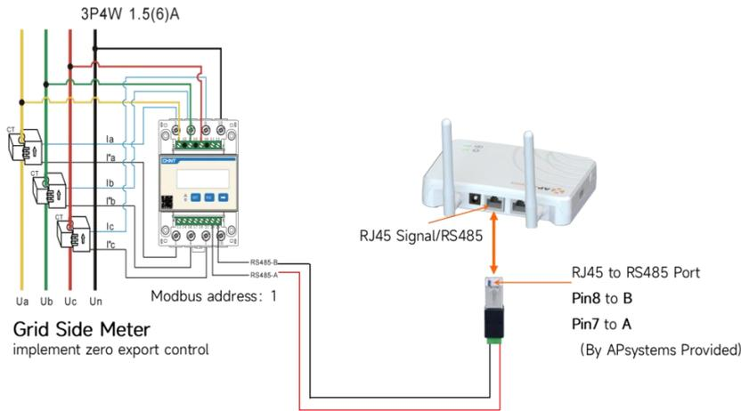
Installation method for Two meters:
