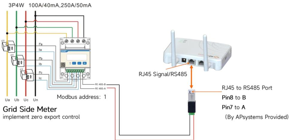
Installation method for Two meters:
