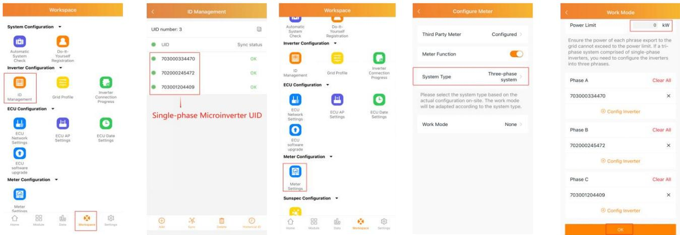
➤ **Single-phase Inverters doing three-phase grid connection, The meter must be of 3P4W(L1-L2-L3-N) type.**
