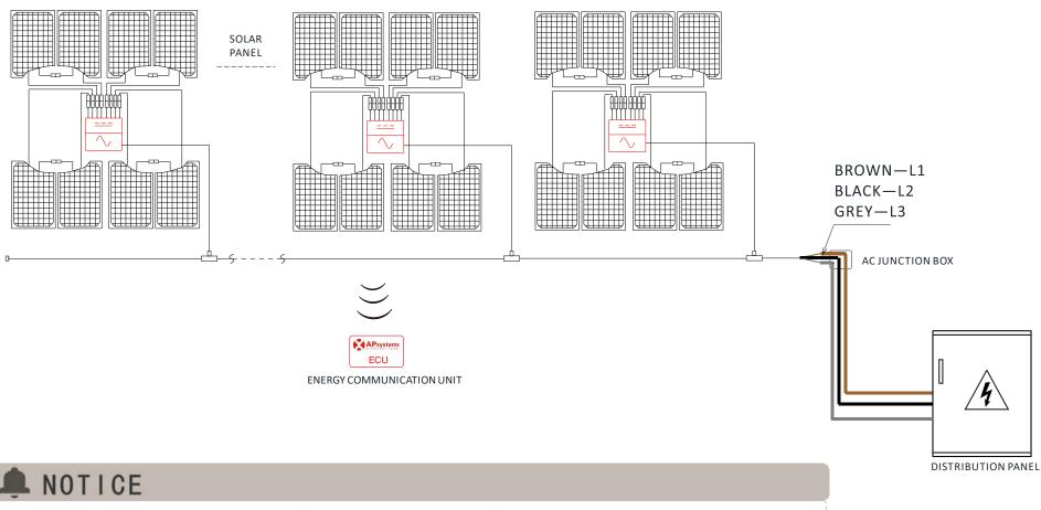
• Each channel connects 2 PV modules in series (For PV modules with Voc<60V). The input channel will not work if connects to a single module(Voc<60V). That means the quantity of PV modules in the sysem is even number.
