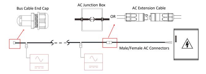
When AC extension cable is needed, users could connect the AC bus cable and AC extension cable in a junction box or use a pair of male/female AC connectors that APsystems provides as optional accessory.
