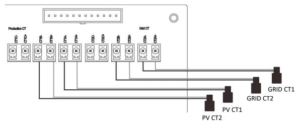
**The direction of CTs:** The arrows on the GRID CT should point from grid to distribution box and the arrows on the PV CT from distribution box to PV.
