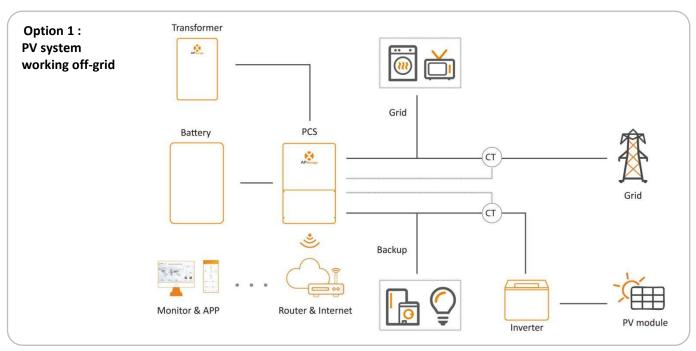
Off grid function only compatible with APsystems DS3 microinverters (fully compatible), as well as QS1 and YC600 microinverters (firmware update required).
