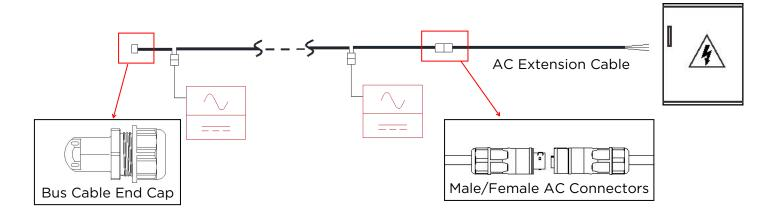
When AC extension cable is needed, users could connect the AC bus cable and AC extension cable in a junction box or use a pair of male/female AC connectors that APsystems provides as optional accessory.
