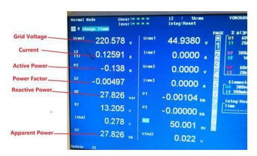
Then the real power consumption in the inverter delivered by following calculations:
