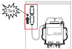
Best Practice: Use the Bus Cable Unlock Tool of AC Bus to disconnect the connectors.
