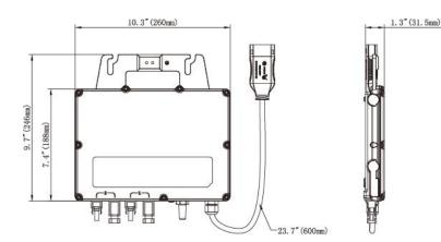
Our flagship new range of Grid-tied microinverters with Reactive Power Control (RPC) features includes the new YC600. The APsystems YC600 is a grid-tied microinverter with intelligent networking and advanced monitoring systems to ensure maximum efficiency. High efficiency, high reliability of the YC600 with 2 independent MPPT inputs, Peak AC output power reaching 600VA. Half the inverters and half the installation means real cost savings for residential and commercial customers.
