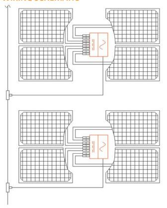
The YC1000-3 is the industry's first true 3-phase solar microinverter, handling commercial grid voltages of 230/400 with 1130 watts maximum output, Wireless communication and an integrated ground. Each YC1000-3 supports up to 4 solar modules.
