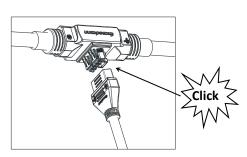
Cover all unused T connectors with Bus Cable T-CONN Cap to protect the T connectors.
