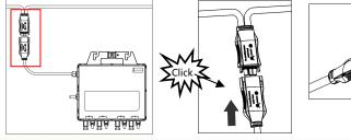
Best Practice: Use the Bus Cable Unlock Tool of AC Bus to split the connectors.
