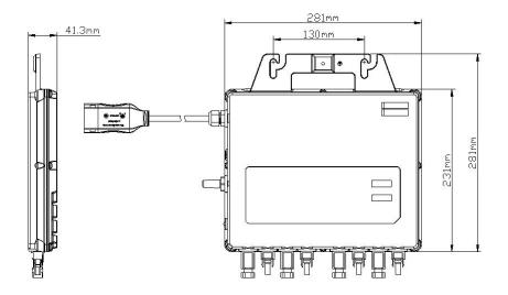
The APsystems QS1 is a grid-tied microinverter with intelligent networking and advanced monitoring systems to ensure maximum efficiency. High efficiency, high reliability of the QS1 with 4 independent MPPT inputs, Maximum AC output power reaching 1200W. Quarter the inverters and quarter the installation means real cost savings for residential and commercial customers.
