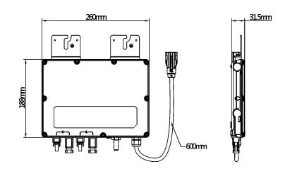
Our flagship new range of Grid-tied microinverters with Reactive Power Control (RPC) features includes the new YC600. The APsystems YC600 is a grid-tied microinverter with intelligent networking and advanced monitoring systems to ensure maximum efficiency. High efficiency, high reliability of the YC600 with 2 independent MPPT inputs, Peak AC output power reaching 600VA. Half the inverters and half the installation means real cost savings for residential and commercial customers.
