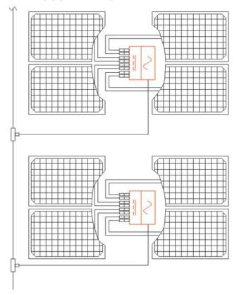
The YC1000-3 is the industry's first true 3-phase solar microinverter, handling commercial grid voltages of 230/400 with 1130 watts maximum output, ZigBee communication and an integrated ground. Each YC1000-3 supports up to 4 solar modules.
