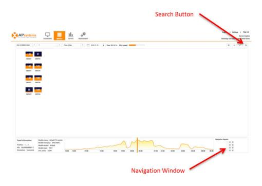
Search Button Allows you find a specific inverter (using its UID) on your array.
