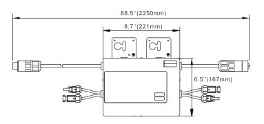
Our flagship product, the APsystems YC500A is a grid-tied microinverter with intelligent networking and monitoring systems to ensure maximum efficiency. Highly dependable and cost effective, the YC500A delivers 250W AC per module with dual MPPT. Half the inverters and half the installation means real cost savings for residential and commercial customers.
