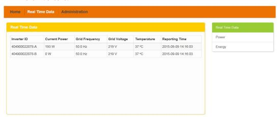
2) If a microinverter does not show up, please confirm if the inverter's ID is correctly input.
