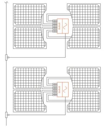
The YC1000-3 is the industry's first true 3-phase solar microinverter, handling commercial grid voltages of 230/400 with 900 watts maximum output, ZigBee communication and an integrated ground. Each YC1000-3 supports up to 4 solar modules.
