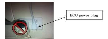
Warning: Do not plug the ECU into a power strip, surge protector, or uninterruptable power supply (UPS). Keep those devices far away from ECU. Those devices can substantially diminish PLC communication performance.
